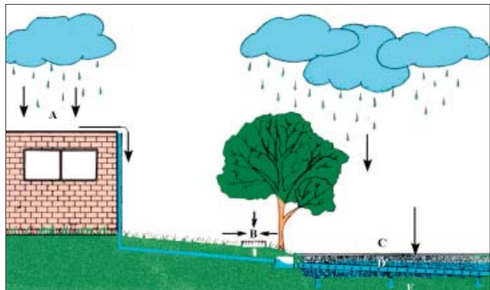
Figure 1. Roof leaders can be connected directly to the subsurface infiltration bed. A) Precipitation is carried from roof by roof drains to storage beds. B) Stormwater runoff from impervious areas and lawn areas is carried to storage beds. C) Precipitation that falls on pervious paving enters storage bed directly. D) Stone beds with 40 percent void space store stormwater. Perforated pipes distribute stormwater from impervious surfaces evenly throughout the beds. E) Stormwater exfiltrates from storage beds into soil and recharges the groundwater. (Cabill Associates Illustration).
